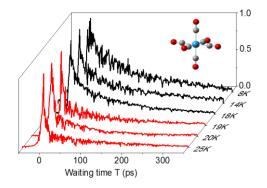
Fig.1 The population dynamics signal of  $W(CO)_6$  isolated in solid methane from 8 K to 25 K. Red – recorded in phase I; black – recorded in phase II. A short component appears in phase I that can be related to a family of sites of high symmetry.
